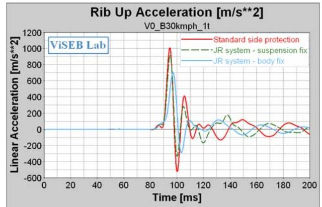
**Figure 7. Rib up acceleration - time history characteristics for three test configurations.**
