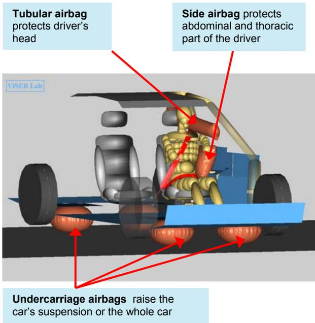
**Figure 2. Elements of the proposed side protection system.**
