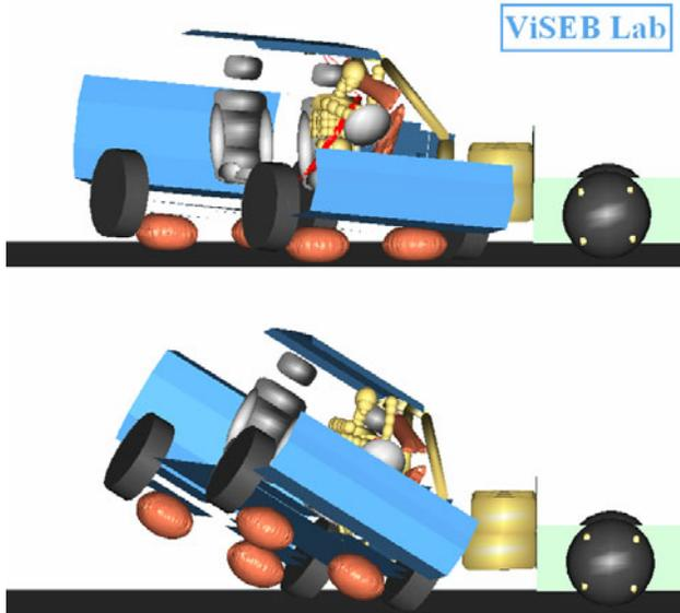
Figure 5. Comparison of the two types of the JR system in 400ms simulation time. Airbags attached to the suspension (upper) and airbags attached to the car body (lower).
