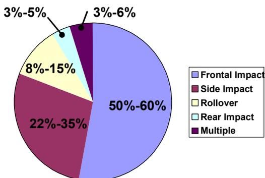
Figure 1. Collision types for car occupant fatalities.
