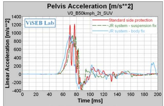
**Figure 6. Pelvis acceleration - time history characteristics for three test configurations.**
